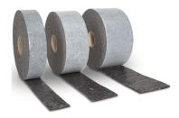
Product description: Sealant tape made of felt, both sides self-adhesive glue based on rubber with protective foil strip. Area of application: For connections of wall and ceiling constructions to adjacent solid components made of concrete or masonry. Suitable for rear connection of Rigips C-wall profiles in double stud walls.
